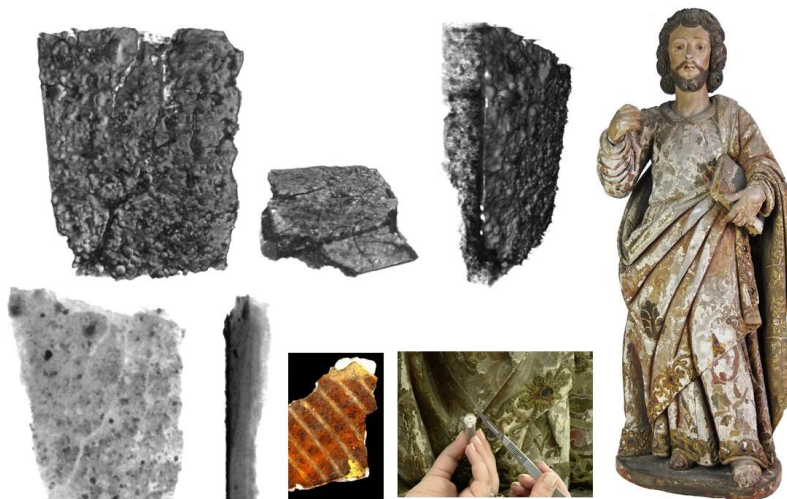
Fig. 1 – Sculpture of St. Joseph, XVI century, Museum of Aveiro. Collecting a gilded polychrome sample PT-SSJ_MA (Gilt Teller Project) in the lower part of the mantle. Microtomographic images (gray images) showing 3D views in partial transparent mode, and two selected radiographs (left bottom).
