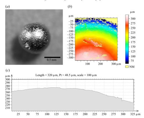
Figure 12. (a) Close-up image of the magnetic sphere with  $D_s = 1$  mm used in the experiments. (b) Surface height distribution measurement results for the sphere with  $D_s = 1$  mm. (c) Surface profile measurement of a part of the same sphere.
