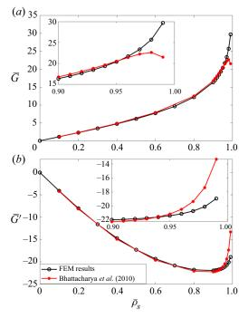
Figure 14. Comparison of the coupling resistance coefficients obtained from the FEM simulations and the data in the literature for  $R_{ch}/R_s=1.6$ . (a)  $\bar{G}$  and (b)  $\bar{G}'$ . The insets show the coefficients for  $\bar{\rho}_s\geq 0.9$ .
