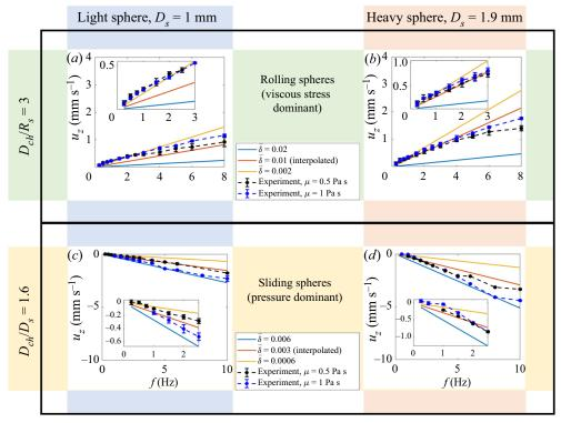
Figure 11. Comparison of  $u_z$  from experiments with the velocities obtained from the resistance coefficients for (a)  $D_s = 1 \text{ mm}$ ,  $D_{ch} = 3 \text{ mm}$ ; (b)  $D_s = 1.9 \text{ mm}$ ,  $D_{ch} = 5.7 \text{ mm}$ ; (c)  $D_s = 1 \text{ mm}$ ,  $D_{ch} = 1.6 \text{ mm}$ ; and (d)  $D_s = 1.9 \text{ mm}$ ,  $D_{ch} = 3 \text{ mm}$ . Insets show  $u_z$  for small f.
