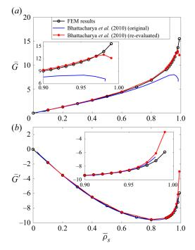
Figure 6. Comparison of the coupling resistance coefficients obtained from the FEM simulations and the data in the literature for  $R_{ch}/R_s = 2$ . (a)  $\bar{G}$ , (b)  $\bar{G}'$ . The insets show the coefficients for  $\bar{\rho}_s \ge 0.9$ .
