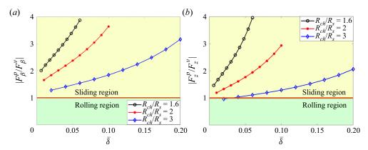
Figure 8. The ratio of magnitudes of viscous and pressure forces contributing to (a)  $\bar{G}(|F_{\beta}^p/F_{\beta}^v|)$  and (b)  $\bar{G}'(|F_z^p/F_z^v|)$ . The subscripts on the terms indicate the direction. The orange lines indicate the transition from sliding to rolling.
