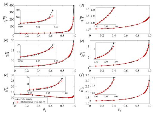
Figure 13. Comparison of the translational and rotational resistance coefficients obtained from the FEM simulations and the data in the literature for  $R_{ch}/R_s=1.6$ . (a)  $\bar{F}^{tt}_{\rho\rho}$ , (b)  $\bar{F}^{tt}_{\beta\beta}$ , (c)  $\bar{F}^{tt}_{zz}$ , (d)  $\bar{F}^{rr}_{\rho\rho}$ , (e)  $\bar{F}^{rr}_{\beta\beta}$  and (f)  $\bar{F}^{rr}_{zz}$ . The insets show the coefficients for  $\bar{\rho}_s \geq 0.9$ .
