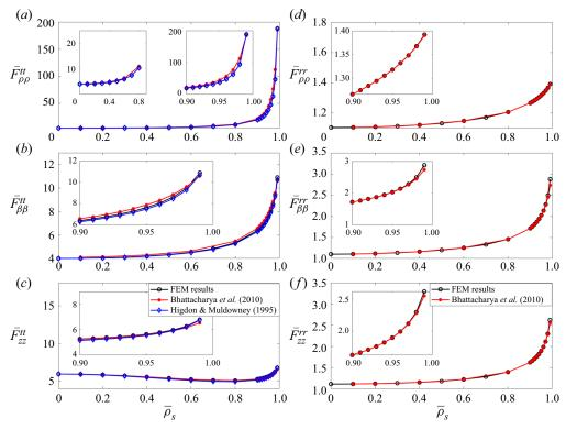
Figure 5. Comparison of the translational and rotational resistance coefficients obtained from the FEM simulations and the data in the literature for  $R_{ch}/R_s=2$ . (a)  $\bar{F}^{tt}_{\rho\rho}$ , (b)  $\bar{F}^{tt}_{\beta\beta}$ , (c)  $\bar{F}^{tt}_{zz}$ , (d)  $\bar{F}^{rr}_{\rho\rho}$ , (e)  $\bar{F}^{rr}_{\beta\beta}$ , and (f)  $\bar{F}^{rr}_{zz}$ . The insets show the coefficients for  $\bar{\rho}_s \geq 0.9$ .
