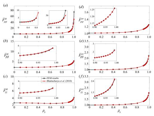
Figure 15. Comparison of the translational and rotational resistance coefficients obtained from the FEM simulations and the data in the literature for  $R_{ch}/R_s=3$ . (a)  $\bar{F}^{rt}_{\rho\rho}$ , (b)  $\bar{F}^{rt}_{\beta\beta}$ , (c)  $\bar{F}^{rt}_{zz}$ , (d)  $\bar{F}^{rr}_{\rho\rho}$ , (e)  $\bar{F}^{rr}_{\beta\beta}$  and (f)  $\bar{F}^{rr}_{zz}$ . The insets show the coefficients for  $\bar{\rho}_s \geq 0.9$ .
