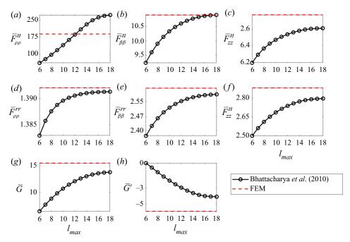
Figure 17. Convergence of the resistance coefficients in the Bhattacharya *et al.* (2010) model for  $R_{ch}/R_s = 2$  and  $\bar{\rho}_s = 0.99$ . (a–c) The translational resistances; (d–f) the rotational resistances; (g,h) the coupling resistances. Finite-element results are shown with dashed lines.
