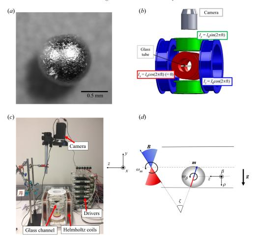
Figure 4. (a) Close-up image of the magnetic sphere with  $D_s = 1$  mm used in the experiments. (b) Schematic drawing of the Helmholtz coil set-up, showing the currents applied to each pair. (c) Experiment set-up for rotating the magnetic spheres. (d) Schematic description of magnetic actuation of the spheres.
