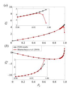
Figure 16. Comparison of the coupling resistance coefficients obtained from the FEM simulations and the data in the literature for  $R_{ch}/R_s = 3$ . (a)  $\bar{G}$  and (b)  $\bar{G}'$ . The insets show the coefficients for  $\bar{\rho}_s \ge 0.9$ .
