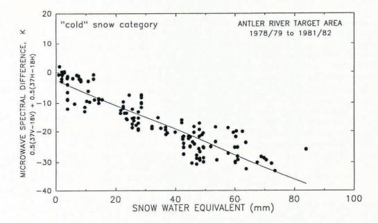
Fig. 3. Linear algorithm for snow water equivalent from Nimbus 7 SMMR observations.
