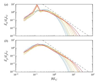
Figure 8. Three-dimensional kinetic and potential energy spectra shown in panels (a) and (b), respectively. The dashed black line indications a -5/3 slope, as assumed by the model spectra (2.16) and (2.15).
