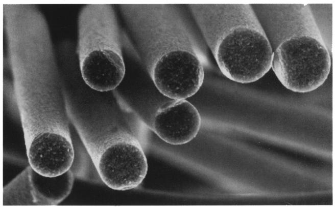
SEM image of superconducting fibers developed at The Washington Technology Center (University of Washington, Seattle, WA) Image acquired by Mike Rock using Gatan's DigiScan" hardware and DigitalMicrograph software.
