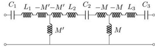
**Fig. 14.** A 1:1 transformer realized with two wireless immittance inverters. At a selected frequency  $\omega = \omega_0$ , the series of  $L_1$ ,  $C_1$ ,  $L_2$ ,  $C_2$ , and  $L_3$ ,  $C_3$  realize short circuits and the entire network behaves as two immittance inverters. When  $M'$  is adjusted to be equal to  $M$ , a 1:1 wireless transformer is realized.
