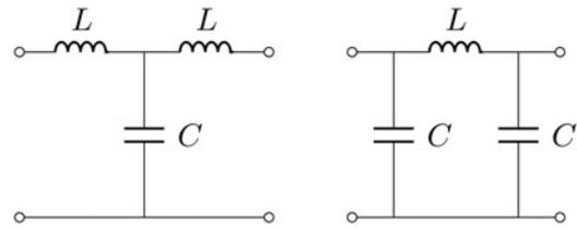
Fig. 7. LC immittance inverters: the Tee( $L, C, L$ ) representation is shown on the left side and provides an inverter value of  $\omega_0 L$ , when equation (7) is satisfied. On the right side is shown a *Pi* network with values  $Pi(C, L, C)$ , which realizes an immittance inverter of value  $\omega_0 L$ .
