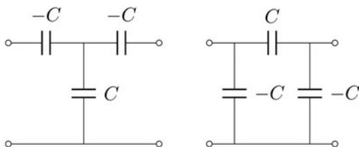
Fig. 6. Capacitive immittance inverters: the Tee representation is shown on the left side and provides an inverter value of  $1/\omega_0 C$ . On the right side is shown a *Pi* network with values  $Pi(-C, C, -C)$  which realizes an immittance inverter of value  $-1/\omega_0 C$ .
