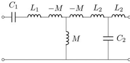
**Fig. 10.** A series capacitance  $C_1$  and a parallel capacitance  $C_2$  have been added respectively on port 1 and port 2. Further addition at port 2 of a series inductor results in the structure shown in the figure. Note that at port 2 the Tee( $L_2$ ,  $C_2$ ,  $L_2$ ) represents another impedance inverter. Thus, at a selected frequency  $\omega = \omega_0$ , the entire network behaves as two cascaded immittance inverters.
