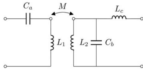
Fig. 3. In this figure  $L_1$  and  $L_2$  are the inductances of the primary and secondary side, respectively;  $M$  is their mutual inductance. A series capacitance  $C_a$  has been added on the primary side; a parallel capacitance  $C_b$  has been added on the secondary side and, finally, a series inductance  $L_c$  has been added on the secondary side. The above network realizes at  $\omega = \omega_0$  a wireless  $1:n$  transformer.
