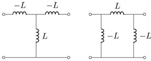
Fig. 5. Inductive immittance inverters: the Tee representation is shown on the left side and provides an inverter value of  $-\omega_0 L$ . On the right side is shown a *Pi* network with values  $Pi(-L, L, -L)$  which realizes an immittance inverter of value  $\omega_0 L$ .
