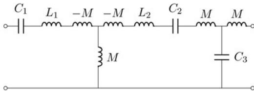
**Fig. 12.** A 1:1 transformer realized with one wireless immittance inverter and one lumped inverter. At a selected frequency  $\omega = \omega_0$ , the series of  $L_1$ ,  $C_1$  and  $L_2$ ,  $C_2$  realize a short circuit and the entire network behaves as two immittance inverters.
