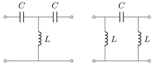
Fig. 8. LC immittance inverters: the Tee( $C, L, C$ ) representation is shown on the left side and provides an inverter value of  $-\omega_0 L$ , when equation (7) is satisfied. On the right side is shown a *Pi* network with values  $Pi(L, C, L)$  which realizes an immittance inverter of value  $-\omega_0 L$ .
