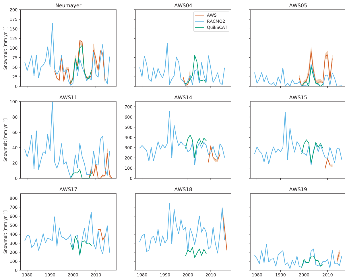
Fig. 6. Time series of in situ melt rate (dark orange), RACMO2 (blue) and QuikSCAT (green). The two in situ melt values for AWS 19 (bottom right) cover only the summer months December–February and November–January respectively, and therefore do not fully capture the melt seasons.
