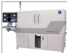
The new ZEISS FPX flat panel extension for the ZEISS Xradia Versa 500-series of 3D x-ray microscopes delivers large-sample, high-throughput scanning. ZEISS Xradia Versa with FPX enables engineering, development, and researchers to scout large samples 2–5× faster to identify a region of interest and
