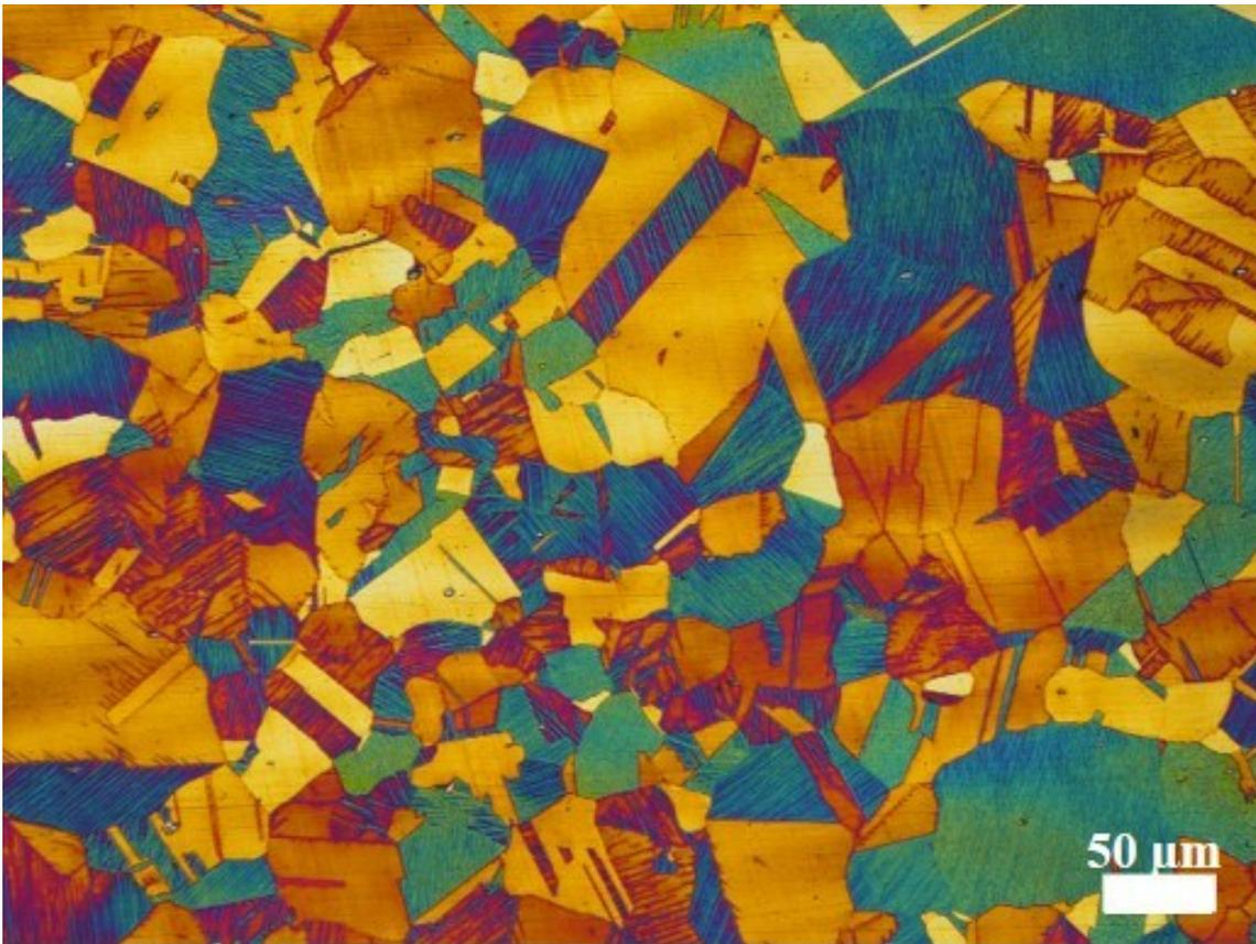
**Figure 2.** Figure 2. Bright field of optical micrographs at 200x magnification in the AISI 304 stainless steel using “aqua regia” ( $\text{HNO}_3+\text{HCl}$ ) and “potassium metabisulfite” ( $\text{K}_2\text{S}_2\text{O}_5$ ) as the chemical etching.
