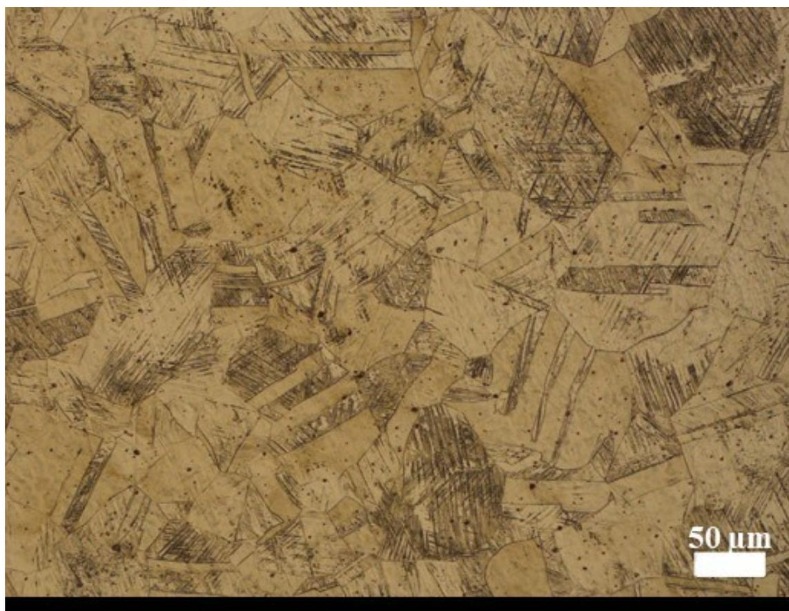
**Figure 1.** Figure 1. Bright field of optical micrographs at 200x magnification in the AISI 304 stainless steel using “aqua regia” ( $\text{HNO}_3+\text{HCl}$ ) as the chemical etching.
