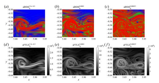
Figure 12. Multiple aBSM (a-c) and aFTLE (d-f) plots for increasing integration times. There is progressively enhanced structural detail as integration time increases, but aBSM and aFTLE ridges become much noisier at the longest integration time, suggesting a saturation in structure information available. Two-component ridges (caps) appear above both vortex heads in regions of low aFTLE at all integration times.
