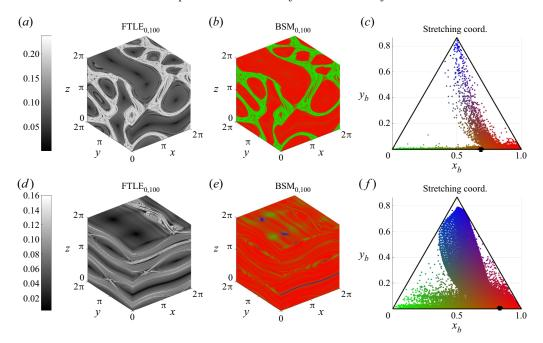
Figure 7. Finite time Lyapunov exponents, BSM and stretching coordinates for the ABC flow: (a-c) A = 1,  $B = \sqrt{2/3}$  and  $C = \sqrt{1/3}$ ; (d-f) A = 1, B = 0.145789 and C = 0.145789.
