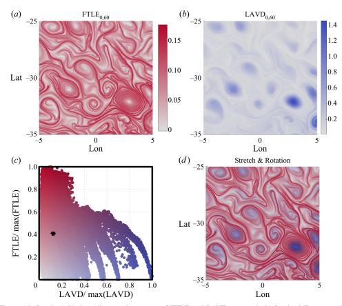
Figure 16. Panels (a,b) show linear colour maps of FTLE and LAVD, respectively for the 2-D geostrophic currents in the Agulhas leakage region. Panel (c) shows the relationship between stretching and rotation for different locations in the flow. Panel (d) combines the stretching and rotation measures to indicate the relative location of fronts and eddies.
