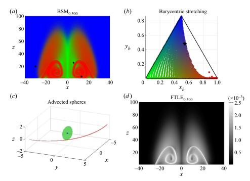
Figure 4. Examining the stationary concentrated vortex structure through the Cauchy–Green eigenvalue BSM (a), stretching coordinates (b), shapes of advected fluid spheres (c) and FTLEs (d).
