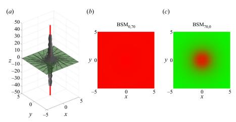
Figure 3. Burgers–Rott vortex streamlines and underlying invariant manifolds (a), forward BSM (b), backward BSM on the z = 0.1 plane (c).
