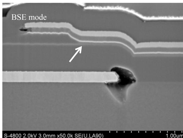
Figure 2. Cross sectional observation of FIB-milled transistor
