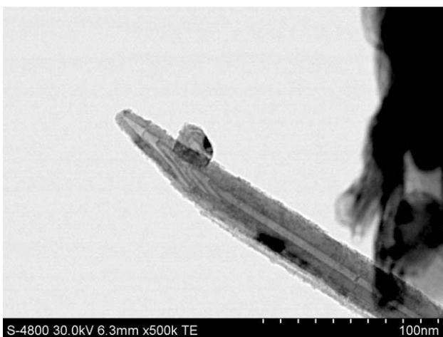
Figure 4. STEM micrograph of multi-layered carbon nanotube
