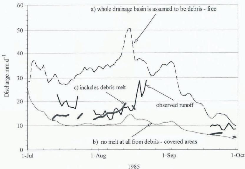
Fig. 6. Comparison of daily observed discharge to simulated runoff in the Lirung drainage basin using the HYCYMODEL, including the melt from the debris zones.
