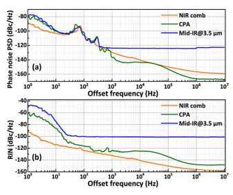
**Figure 5.** (a) Phase noise PSD and (b) relative intensity noise (RIN) of the repetition rate signal corresponding to NIR comb (origin), CPA (green), and mid-IR comb at  $3.5 \mu m$  (blue).
