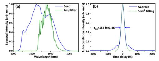
**Figure 2.** Characterization of the chirped pulse amplification. (a) Normalized optical spectrum of NIR oscillator (blue curve) and amplified pulse (green line), centered at 1030 and 1038 nm with a spectral width of 30 and 12 nm, respectively. (b) Measured autocorrelation trace (blue line) of the amplified pulse with corresponding sech fitting (dotted green line).
