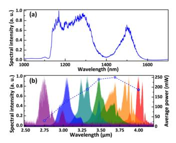
**Figure 3.** (a) The spectrum of the broadened signal laser after a long-pass filter at 1100 nm. (b) The spectrum and corresponding average power of the mid-IR comb. The mid-IR comb has a tunable coverage of  $2.7–4.0~\mu m$ . The average powers are 30, 130, 190, 240, 250, and 187 mW centered at 2.7, 3.0, 3.3, 3.5, 3.7, and 4.0  $\mu m$ , respectively.
