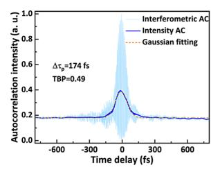
**Figure 4.** The autocorrelation of mid-IR pulse at 3.5  $\mu m$ . The pulse duration is 174 fs with Gaussian fitting.
