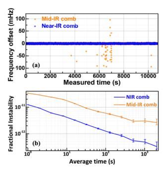
**Figure 6.** (a) The measured repetition rate stability of NIR comb (blue) and mid-IR comb (orange) for 3 h. (b) The Allan variance of the NIR comb (blue) and mid-IR comb (orange).
