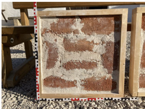
Figure 3. Framed bricks, onto which we applied our experimental mortars.
