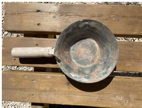
Figure 4. Builder's scoop (capacity: 0.7 l) used for our measurements.
