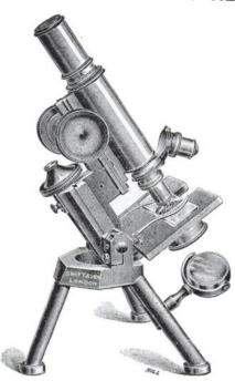
with coarse adjustment by rack and pinion, fine adjustment by micrometer screw, 2/3'' and 1/6'' objectives, one ocular and iris diaphragm, in Cabinet... 26 155.
