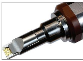
Hummingbird Scientific's new *in situ* TEM MEMS Heating + Biasing Specimen Holder allows users to heat and/or electrically bias samples inside the TEM. Heating can be performed to temperatures  $> 1000^{\circ}\text{C}$ . MEMS chips are directly inserted into the holder via a proprietary 9-pin connector. The holder is available in both single and double-tilt configurations.
