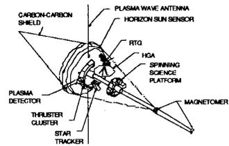
Figure 3. The Solar Probe spacecraft configuration.
