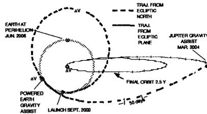
Figure 1. The Solar Probe Trajectory
