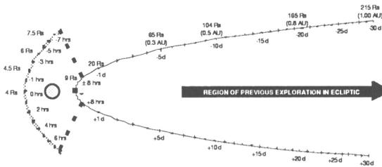
Figure 2. The near perihelion trajectory. The orbit plane is orthogonal to the Earth-Sun line.
