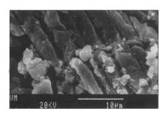
Figure 2. A scanning electron micrograph of a deteriorated calcite crystal (in marble), split open along its cleavage planes.
