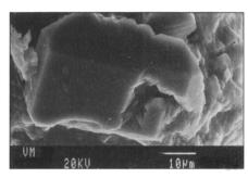
Figure 4. An affected quartz crystal in the sandstone. Its edges have been corroded, and part of it has decomposed.
