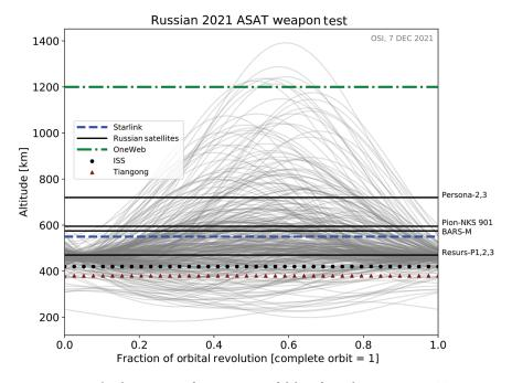
**Figure 7.3** Orbital trajectories for 340 pieces of debris from the Russian ASAT weapon test. The debris fragments cover a large range of low Earth orbits, crossing critical infrastructure, including the ISS, the Tiangong Space station and Russian satellites. Moreover, due to the high altitude of the test, all of the debris fragments will pass through the orbital space of the ISS and the Tiangong Space station as they decay.
