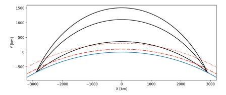
**Figure 7.5** Ballistic trajectories for three different profiles, showing a depressed, an efficient and a high-altitude trajectory. The blue curve represents the surface of the Earth, while the dot-dashed curve is at an altitude of 100 kilometres and the dotted line is at 300 kilometres.
