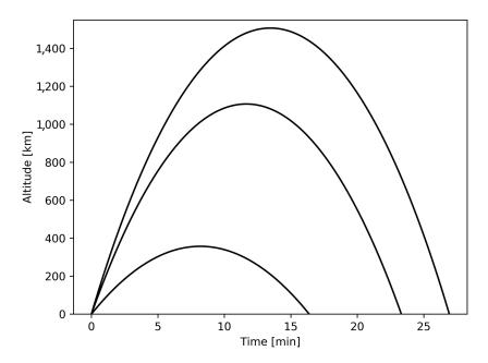
**Figure 7.6** Simplified example of the flight times corresponding to the depressed, efficient and high-altitude trajectories in Figure 7.5. The times are based on Keplerian arcs, so they do not account for the time needed to accelerate the ICBMs to burnout (at around 100 kilometres). Nonetheless, this introduces a timing difference of only one to a few minutes, so the overall scale of the flight times is preserved.
