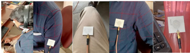
Figure 24. Real-time on-body measurement setup.
