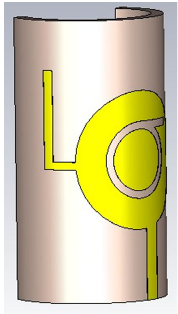
Figure 20. Antenna bent in y orientation.
