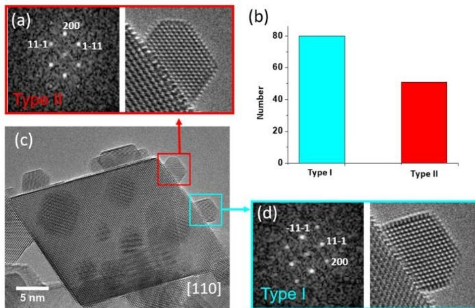
**Figure 1.** Typical morphology of the as-received Au/CeO<sub>2</sub> sample along with the occurrence of the two states.
