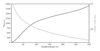
**Figure 1.** The number of MWA baselines shorter than a given length (solid line) for a zenith pointing. The dotted grey line indicates the spatial scale that a given baseline is sensitive to.
