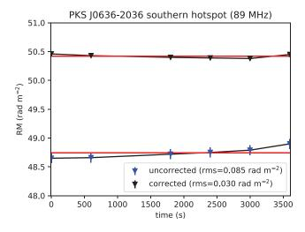
**Figure 10.** Variation in observed rotation measure in the southern hotspot of PKS J0636–2036 as a function of time in the lowest MWA band (89 MHz). Blue points show the measured RM before ionospheric calibration and the Black points show the measured RM after ionospheric calibration. The red line shows the mean value of RM in each instance.
