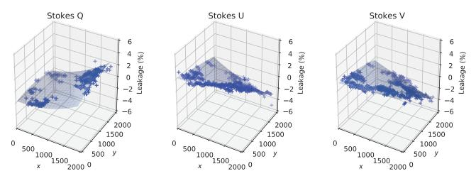
**Figure 6.** A sample demonstrating the fitting of point-source leakage over the observed field-of-view. The points were taken from one of the beamformer pointings used during a 'drift and shift' observation. Fits were performed separately for different beamformer pointings and for each of the different Stokes parameters (Q, U, and V). The X and Y axis are in units of pixels for a  $25^{\circ} \times 25^{\circ}$  field.
