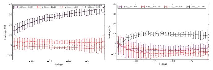
**Figure 5.** Left: Declination-dependent leakage observed in the MWA 216 MHz band for a  $\delta = -13^{\circ}$  declination meridian scan using an analytic beam model to correct for instrumental polarisation. The plot shows the median fractional polarisation for Stokes Q, U, and V where q = Q/I, u = U/I and v = V/I. The fractional linearly polarised intensity p is also shown where  $p = \sqrt{Q^2 + U^2}/I$ . Right: Same as left but using the Sutinjo et al. (2015) beam model.
