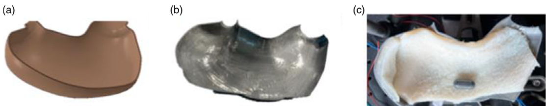
Figure 11. (a) CAD drawing of the stomach phantom, (b) 3D-printed PLA phantom, and (c) bovine stomach paved on the stomach phantom.
