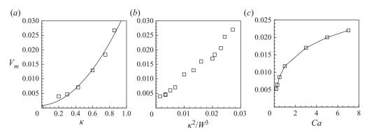
Figure 6. Migration velocity near the curved channel centre as a function of  $(a) \kappa$ ,  $(b) \kappa^2/W^3$  and (c) Ca.
