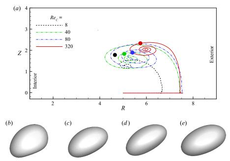
Figure 14. Migration of a capsule toward the vortex centre. (a) Influence of  $Re_C$  on capsule trajectory and equilibrium location in comparison with the location of the vortex centre is shown for  $R_C = 5$ , W = H = 4. Filled circles indicate the vortex centre for  $Re_C = 8$  (black), 40 (green), 80 (blue), 320 (red). (b–e) Capsule shapes near respective equilibrium locations for different  $Re_C$ ; (b)  $Re_C = 0.8$ , (c)  $Re_C = 2$ , (d)  $Re_C = 8$  and (e)  $Re_C = 80$ .
