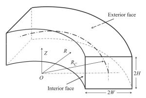
Figure 1. Schematic of a curved microchannel of rectangular cross-section. All lengths are shown in dimensionless form scaled by capsule radius. Channel centreline (radius of curvature  $R_C$ ) is indicated by a dash-dot curve.
