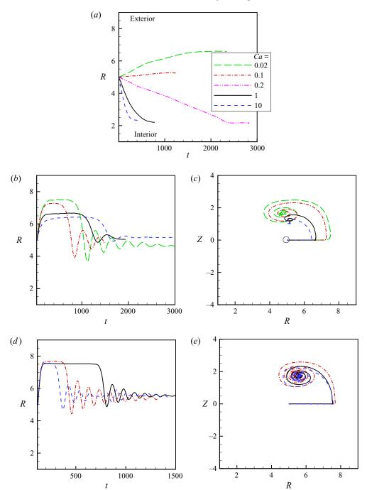
Figure 16. Effect of capsule deformability in the inertial regime. Trajectories are shown at different Ca by considering a weaker secondary flow in (a) for  $Re_C = 0.8$ , and stronger secondary flows in (b,c) for  $Re_C = 8$ , and in (d,e) for  $Re_C = 80$ . Line symbols for different Ca are same for all plots and indicated in (a). Radial trajectories versus time are shown in (a,b,d), while cross-sectional trajectories are shown in (c,e).
