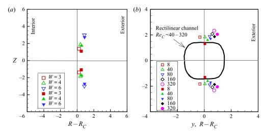
Figure 17. (a) Influence of channel width (square cross-section) on vortex centres (open symbols) and capsule equilibrium locations (filled symbols). Here  $R_C = 7$  is fixed. (b) Comparison of equilibrium locations in a curved channel ( $R_C = 5$ ) and in a rectilinear channel of the same W = H = 4. For the rectilinear channel, the equilibrium locations lie on a squircle as indicated, whereas they are unique locations for the curved channel.
