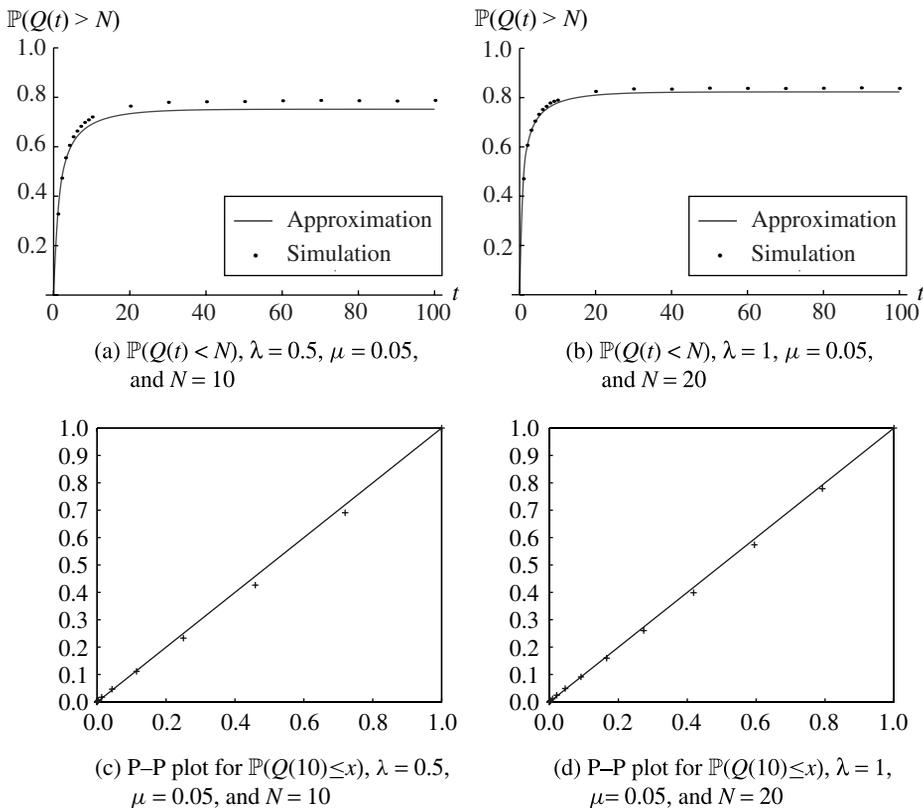
FIGURE 3: Simulated and approximated results for the M/M/N/N queueing model.
