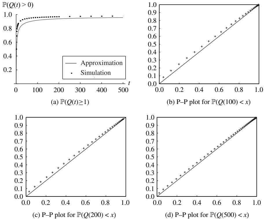
FIGURE 2: Simulated and approximated results for the GI/GI/1+GI queueing model when the interarrival and service time distributions are gamma(2,2) and the reneging distribution  $F$  is uniform on  $[0, 1000]$ .
