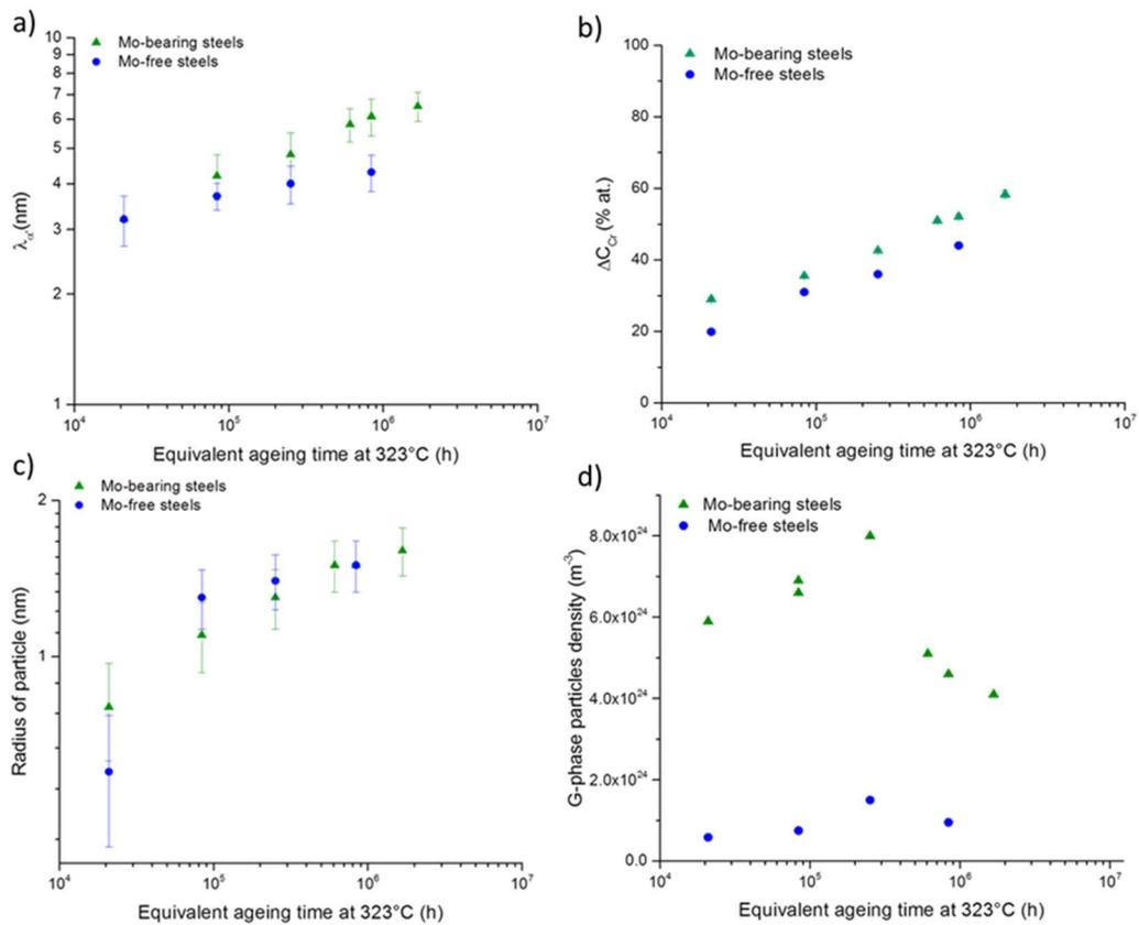
**Figure 2.** Time evolution of the mean wavelength (a), and amplitude of Cr concentration (b) of the spinodal decomposition, evolution of the radius (c), and the number density (d) of G phase particles in the ferrite of Mo-bearing steels, green triangle, and Mo-free steel, blue circles.
