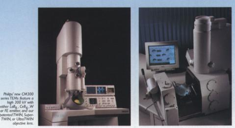
The new XL40 FEG SEM features a 150 mm motorized eucentric stage, conical end-lens and large chamber with full system automation and integrated image anabeis
