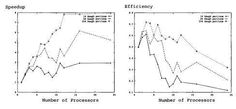
Fig. 11. Performance of the Occam2 Hough implementation
