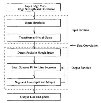
Fig. 3. Block diagram of the Hough implementation
