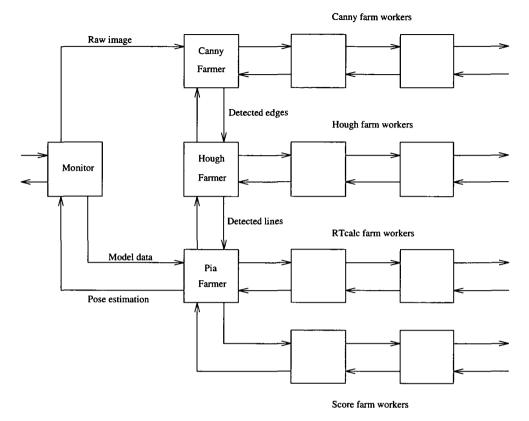
Fig. 20. The architecture of the object recognition system
