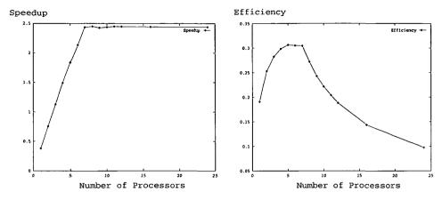
Fig. 21. Performance of the Occam2 Canny implementation
