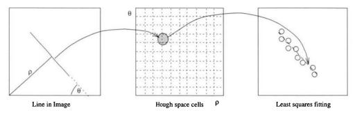
Fig. 2. Schematic of the Hough transform process
