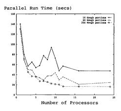
Fig. 10. Parallel execution time for the Occam2 Hough implementation
