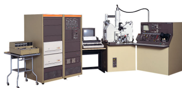
FIG. 2. JXA-733 and trace elemental mapping results (Dendrite structure of P, Si in a Steel).
