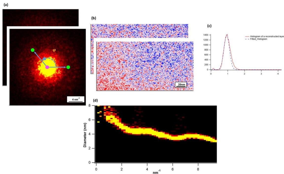
**Figure 2.** Figure 2. (a) layers of a-BC:H nano-diffraction patterns, (b) reconstructed images of nano-diffractions at one  $k$  and  $\phi$  with visible speckles, (c) a typical histogram of intensities in a reconstructed image, and (d) a 2D histogram of distribution of MROs sizes as a function  $k$  vector.
