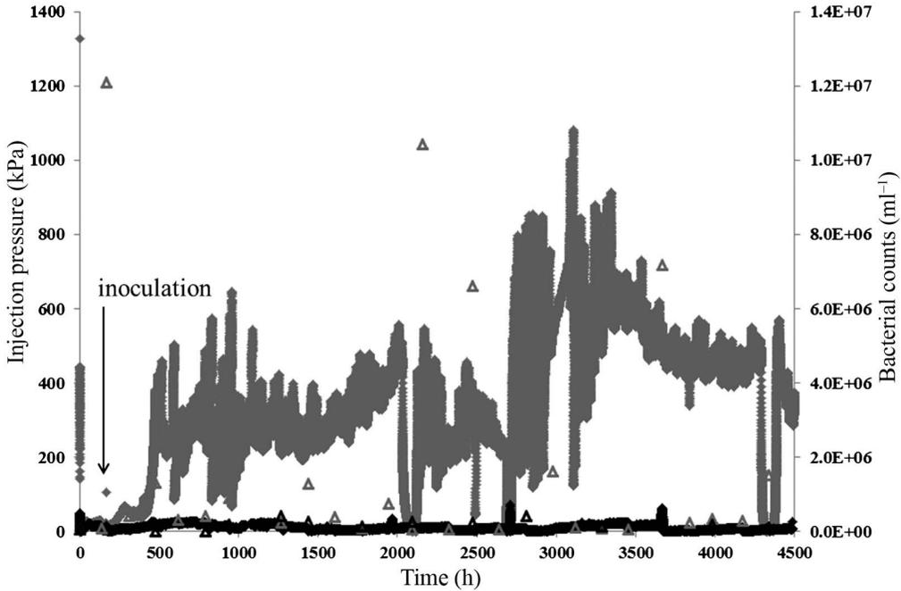
FIG. 2. Injection pressure and bacterial count data for the control and biotic sandstone column experiments. The control pressure and bacterial counts are shown by a black line and black open triangles, respectively. The biotic pressure and bacterial counts are shown by a grey line and grey open triangles, respectively.
