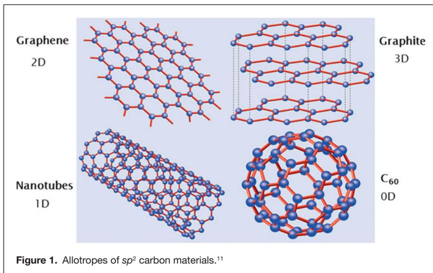
Figure 1. Allotropes of  $sp^2$  carbon materials.<sup>11</sup>
