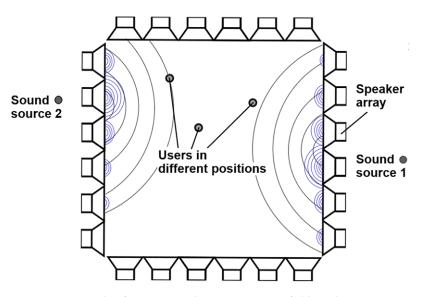
**Figure 17.** Principle of acoustic rendering using wave-field synthesis; two (external) sound sources as an example; source: (Husung 2012), edited and translated into English by the authors.
