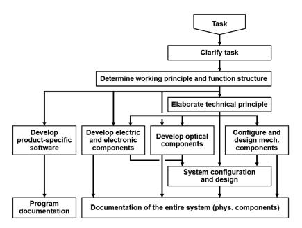
**Figure 11.** Model of the development and design process for precision engineering and mechatronic products; outcome of the MAKON project (Höhne *et al.* 1983); translated into English by the authors.
