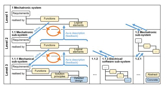
**Figure 31.** Interactions at the different levels of the system (Husung *et al.* 2022*b*), expanded on the basis of Pohl *et al.* (2012).
