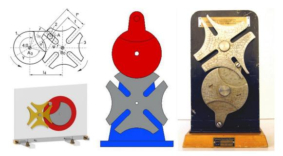
**Figure 15.** Step mechanism of the Geneva type (Maltese cross mechanism), excerpt of DMG-Lib (www.dmg-lib.org): drawing [RWTH Aachen], plastic model for teaching [RWTH Aachen], CAD model [Universitatea Politehnica Timisoara], metal model manufactured 1930 [TU Dresden]. In DMG-Lib all models, except the drawing, can be animated, in video as well as interactive forms.
