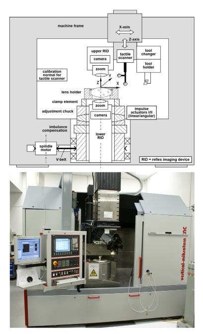
**Figure 12.** Self-adjusting alignment turning station for centring and aligning mounted lenses (Frank 2008); top – technical principle, translated into English by the authors; bottom – machine as built and used [Carl Zeiss Jena GmbH].
