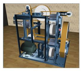
**Figure 23.** Pick-and-place machine – example of a virtual assembly including acoustics.
