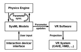
**Figure 26.** Flow of information between different tools during VR simulation (Mahboob *et al.* 2019*a*).
