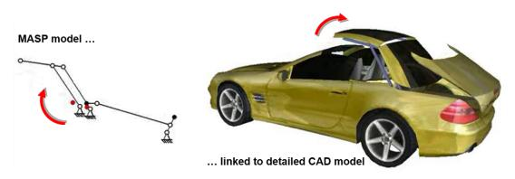
**Figure 14.** Modelling of a mechanism with MASP (Modelling and Analysis of Solution Principles) and link to a fully detailed CAD model (example after Höhne *et al.* 2005*b*).
