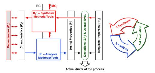
Figure 28. The product development/design process scheme according to the CPM/PDD approach.
