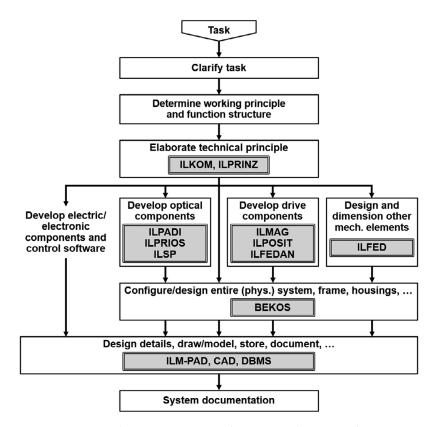
**Figure 13.** ILKON (ILmenauer KONstruktionssystem), a comprehensive computer support system to assist the design of precision engineering and mechatronic products, based on results of the MAKON project (see Figure 11), developed in cooperation with other groups at TH Ilmenau (Höhne 1990); scheme translated into English by the authors.
