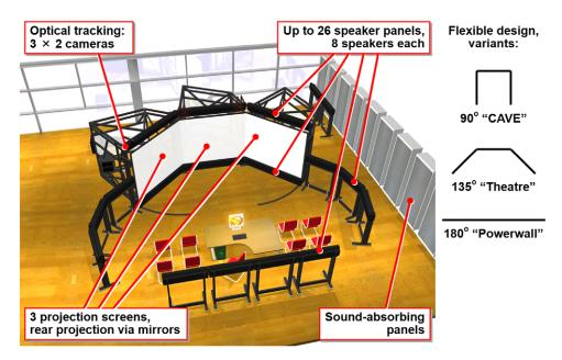
**Figure 16.** Flexible Audio-Visual Stereo Projection Device (FASP) at TU Ilmenau; visualisation by three stereo projection screens in flexible configurations, auralisation (acoustic presentation) via Wave-Field Synthesis (WFS) produced by speaker panels arranged in a plane roughly at the height of the users' ears.
