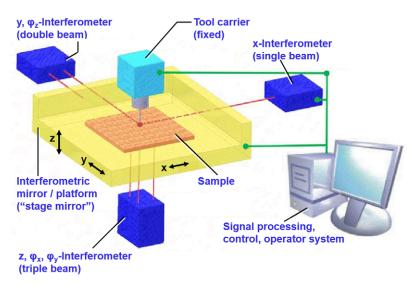
**Figure 18.** Working Principle of the Nanopositioning and Nanomeasuring Machine (NPMM), based on Jäger *et al.* (2009).
