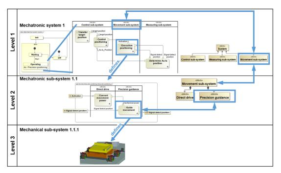
Figure 30. Top-down approach with the distribution of the required sub-functions to the sub-systems (Husung *et al.* 2022*b*).
