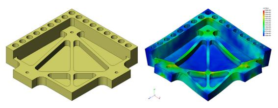
**Figure 20.** Optimised interferometric mirror ("stage mirror") of the Nanopositioning and Nanomeasuring Machine; CAD-model and simulation (Lotz 2009).
