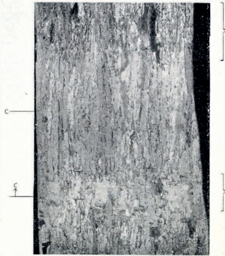
Fig. 6. Banded sea ice. Upper bracketed zone is the white band corresponding to the 4 in. to 5 in. zone in Figure 3; lower columnar crystal zone is the 6.5 in. to 7 in. vertical c -axis band. Note terminal brine pockets associated with the c -axis vertical crystals. Vertical section 6 cm. \times 10 cm. Between crossed polaroids
