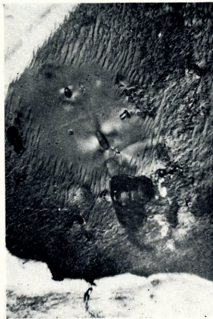
Fig. 17. Horizontal thin section of sea ice. Pressure shadows from internal stress developed by expanding brine pockets clearly expressed. \times 50 between crossed Nicols
