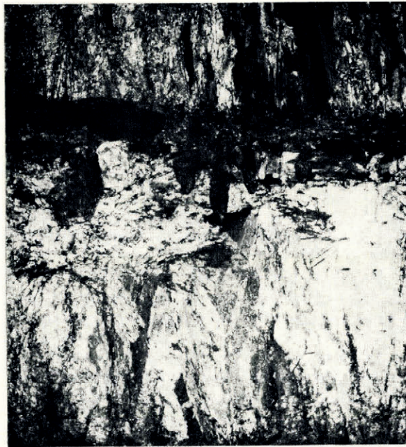
Fig. 1. Brine drainage features in natural sea ice. Ice 8 cm. thick from recently frozen lead. Top of specimen is sea-ice surface, bottom of specimen is sea-ice-water interface. Note "funnel" shaped platelet orientation feature from brine drainage. Brine corrosion pockets observable below thrust band. Vertical thin section is 4 mm. thick. Between crossed polaroids
