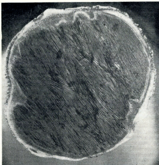
Fig. 11. Horizontal thin section from 3 in. (7.6 cm.) core cut 3 cm. above ice-water interface. Black areas are drainage channels. Note intergrowths. Double exposure of fluorescein-dyed specimen. Thickness of specimen conceals effect of crossed polaroids. Maximum ice section diameter is 3 in. (7.6 cm.). Fringe around platelet area is ice from pure water applied as "cement"
