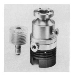
Turbomolecular Pump: High-performance Turbovac 50 with DN35CF flange eliminates flange adaptors and reduces space requirements. Features include modular single-unit construction, low vibration, quiet operation, and low maintenance. Normal operating temperature up to 35°C requires no additional cooling; air or water cooling is optional. Leybold Vacuum Products Inc., 5700 Mellon Road, Export, PA 15632; (412) 327-5700.
