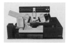
The single-cassette, random access system handles 100 mm, 125 mm, or 150 mm samples without use of belts or air track. It can be ordered as an AutoEL option or a retrofit for existing systems. Rudolph Research, One Rudolph Road, Box 1000, Flanders, NJ 07836; (201) 691-1300.
