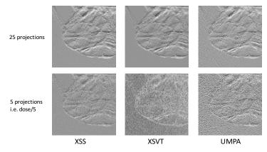
**Figure. 1.** XY differential phase contrast map obtained with XSS, XSVT and UMPA method of a fly phantom using a parallel beam at 3.5μm and reconstructed with 25 points or 5 points on the sample.
