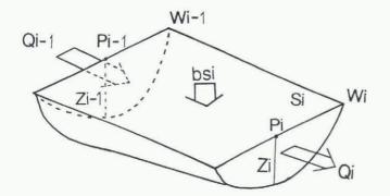
Fig. 4. A section of the glacier, as defined by the model with the symbols in the text. Glacier AX010 is divided into eight such sections (i: 1-8).
