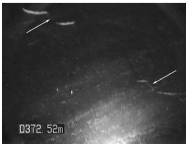
Fig. 10. Pairs of brine cells joined by steps (arrowed) to form larger brine inclusions, with brine channels also becoming prevalent from around this depth.
