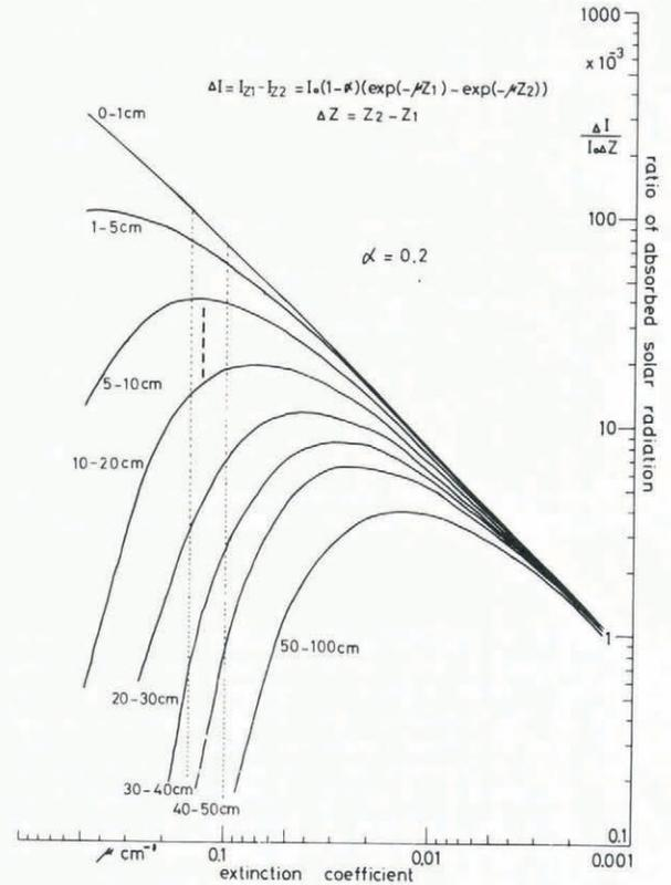
Fig.5. Ratios of absorbed radiation amounts at a unit volume to the incident solar radiation with relation to extinction coefficient. parameter: albedo
