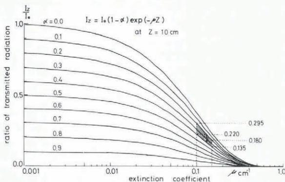
Fig.4. Ratios of the transmitted radiation to the incident solar radiation with relation to extinction coefficient. parameter: albedo
