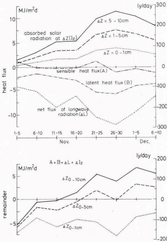
Fig.6. Daily means of heat balance components at layer  $\Delta Z$ , and remainder term of Equation 3 averaged for 5 days.
