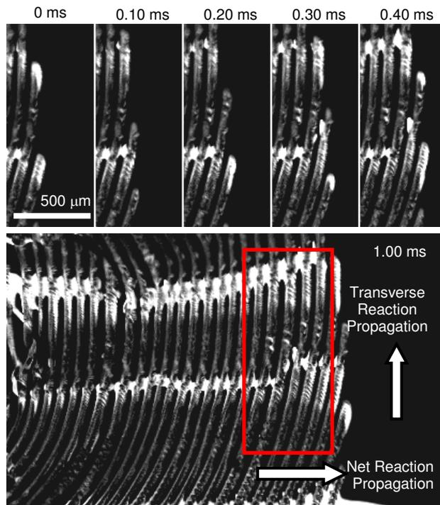
**FIG 2.** Still frame captures from a high speed movie of an exothermic reaction in a Sc/Cu foil with 41.2 nm bilayer thickness. The time stamp in/above each image is relative to the first image in the sequence, while the scale bar in the upper left image applies to all images. Note that external illumination was used and the contrast apparent in the images is strictly reflected light.
