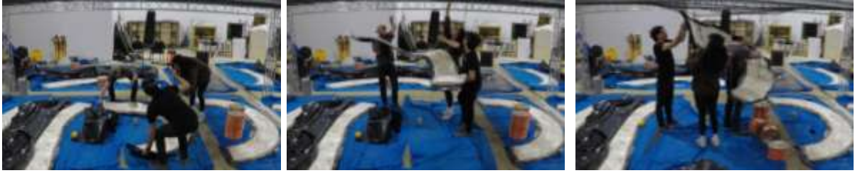
Figure 7. In step 3, the cultivated sheets are hang-dried into their 3D form. Photos by Jonathan Dessi-Olive.
