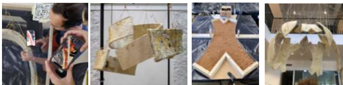
Figure 2. Processes and prototypes that preceded the design, cultivation, and installation of Phoenix. On the left, bending living sheets guided by augmented reality for the Myco-Chandelier. On the right, cultivating non-rectangular sheets with flexible formwork for the hanging Myco-Pod. Photos by Jonathan Dessi-Olive.
