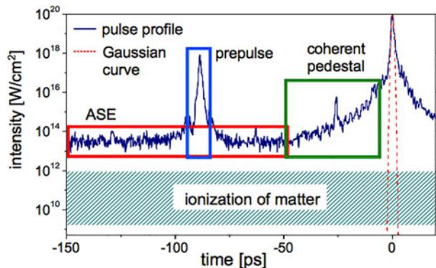
**Figure 1.** Temporal profile of the PHELIX pulse in 2010 before the application of pulse cleaning techniques, measured with a third order cross-correlator (Sequoia, Amplitude Technologies). The curve has been scaled to a peak intensity of  $10^{20} \text{ W cm}^{-2}$ . The shaded area illustrates the ionization threshold for typical target materials. The red dashed line shows a Gaussian function with the same FWHM as the pulse (blue).
