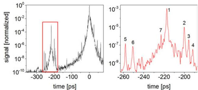
**Figure 4.** Temporal profile of the PHELIX pulse in 2012 using the uOPA with a gain of  $10^4$ . The pulse was measured with a third order cross-correlator (Sequoia, Amplitude Technologies). The right graph shows an enlargement of the red framed region of the left graph.
