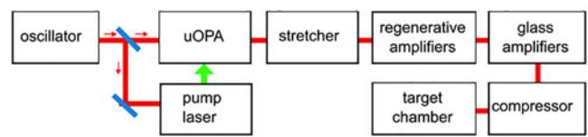
**Figure 3.** Schematic of the PHELIX short pulse beamline.
