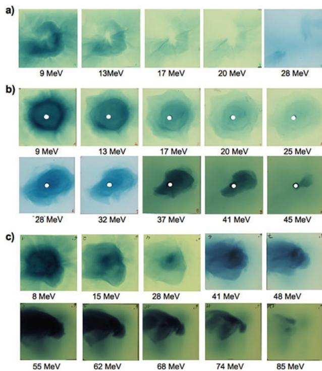
**Figure 8.** Selection of RCF which were exposed to laser-accelerated proton beams. The energy of protons which are fully stopped in the particular foil are written underneath each layer. Shown are examples for: (a) a shot with a ns-prepulse with a contrast ratio around  $10^6$ , (b) a shot after removing the prepulse and (c) a shot using the full aberration control.
