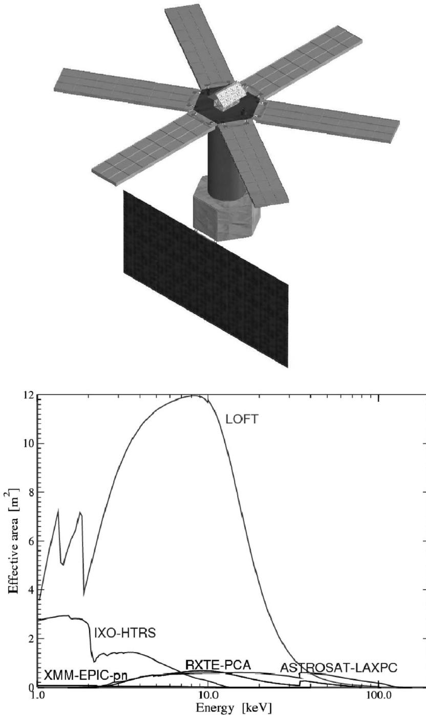
**Figure 1.** Upper: Conceptual scheme of the *LOFT* satellite. From top to bottom along the satellite axis: Wide Field Monitor, optical bench, the six Large Area Detector petals, structural tower, bus, and solar array. Lower: LAD effective area plotted against energy in linear scale, as compared to that of other satellites for X-ray astronomy (from Feroci *et al.* 2011a)
