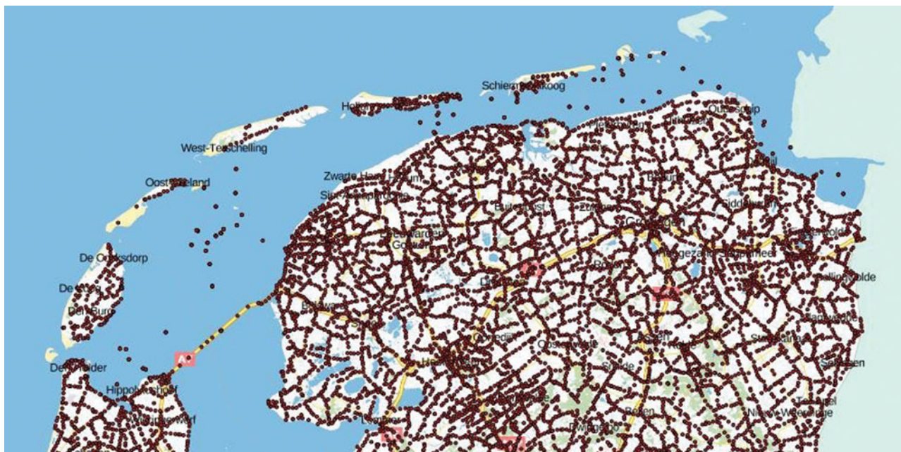
Fig. 26. Location of the NAP benchmarks in the Wadden Sea area. For each benchmark, the latest surveyed NAP height and the location of the benchmark is given. From http://pdokviewer.pdok.nl/ , visited 12 September 2017.
