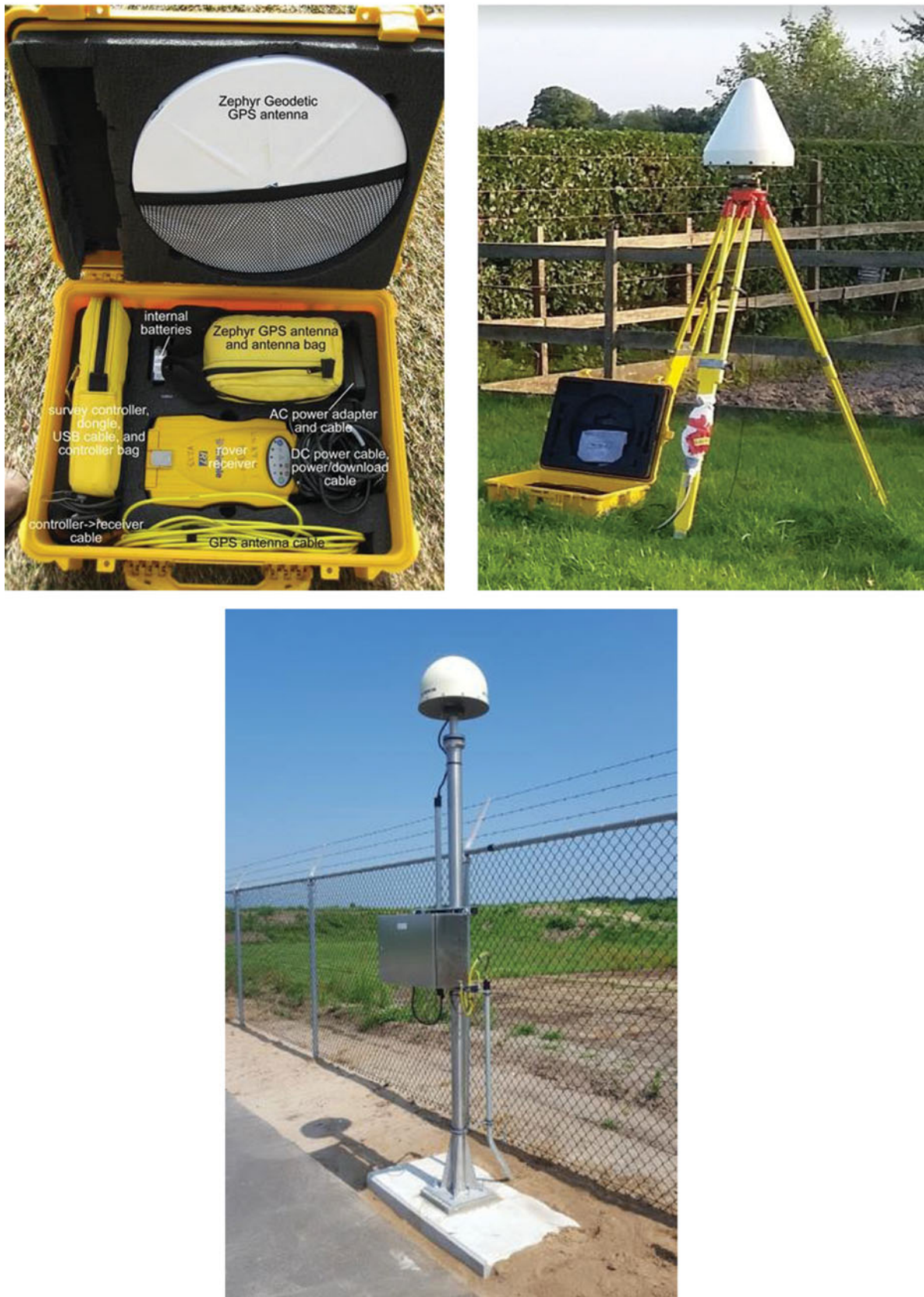
Fig. 12. Three examples of a geodetic receiver unit. On the left a campaign receiver and antenna in a case with all accessories (image courtesy UNAVCO), in the middle a typical field set-up with antenna on a tripod centred above a marker and battery-powered receiver in the waterproof case (data are stored on a flash card inside the receiver) (image TU Delft), and on the right a Continuous Operating Reference Station (CORS) from NAM, with receiver and data modem inside the cabinet (image courtesy O6-GPS).
