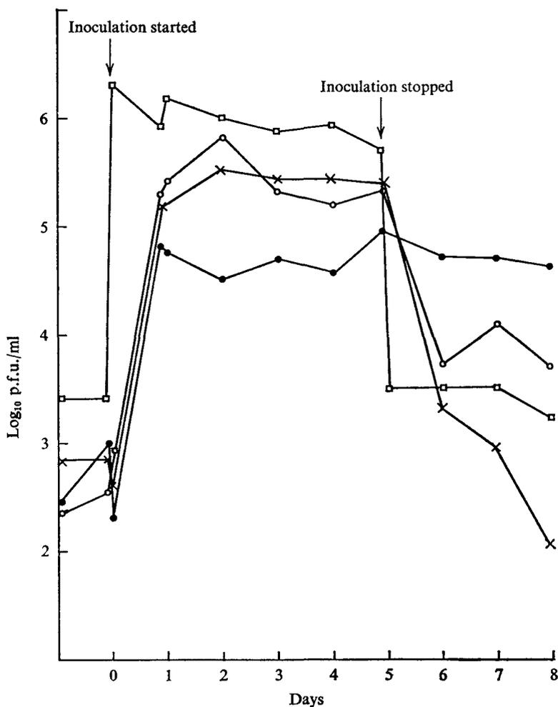
Fig. 1. Distribution of virus in the model plant before, during and after cessation of inoculation with virus. Virus in raw settled sewage (□—□), effluent (×—×), mixed liquor liquid fraction (○—○) and mixed liquor solids fraction (●—●).
