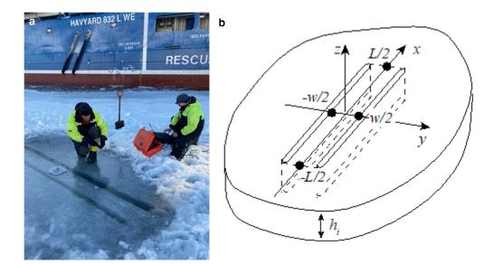
Figure 2. (a) Fixed-ends beam in landfast ice of Tempelfjorden. (b) Schematic of the test with vibrating floating fixed-ends beam.
