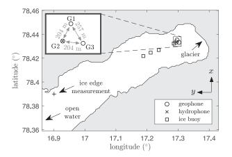
**Figure 1.** Experimental setup in Tempelfjorden, Svalbard. Instrument deployment consists of three geophone logger (also see inset), a hydrophone and four wave-ice buoys. In situ cantilever experiments were performed near the ice edge, marked by the '+' sign.
