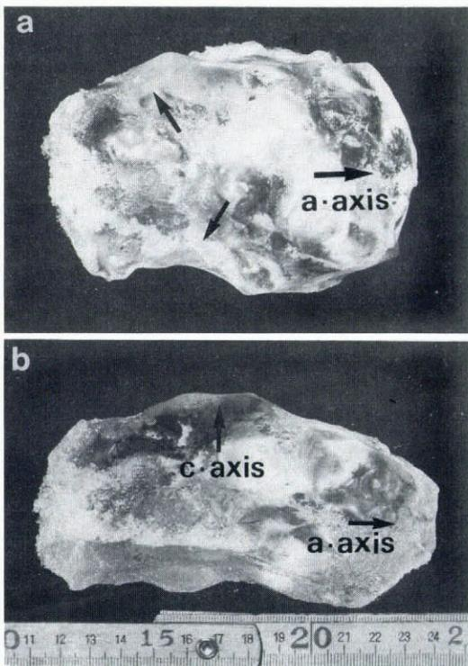
Fig. 2. Photographs of a large-sized single crystal of ice from Mendenhall Glacier with the crystallographic axes denoted by arrows; a: view from above; b: side view.
