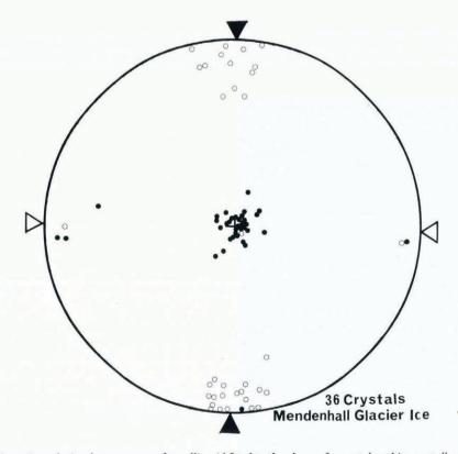
Fig. 3. Orientation relation between axes of an ellipsoid fitted to the shape of a crystal and its crystallographic axes in a stereographic projection with the shortest axis of the ellipsoid as centre. ▲: direction of the longest axis of the ellipsoid. △: direction of the middle axis of the ellipsoid. ◆: orientation of the c-axis of the crystal. ○: orientation of one of the a-axes of the crystal.
