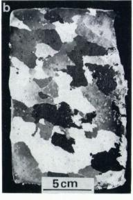
Fig. 4. Photographs of thin sections of a Cape Folger core ice sample at a depth of 324 m taken under crossed polaroids; a: horizontal thin section; b: vertical thin section.
