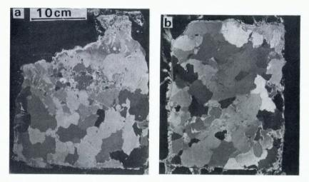
Fig. 1. Polarized photographs of thin sections of a Mendenhall Glacier ice sample cut out from an iceberg where large-sized crystals were collected. The two sections intersected at right angles; a: face A; b: face D.
