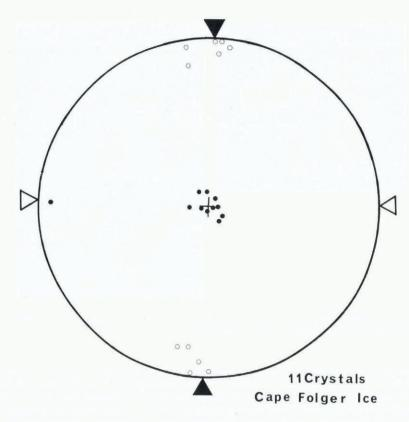
Fig. 5. Orientation relation between axes of an ellipsoid fitted to the shape of a crystal and its crystallographic axes in a stereographic projection with the shortest axis of the ellipsoid as centre. ▲: direction of the longest axis of the ellipsoid. △: direction of the middle axis of the ellipsoid. ◆: orientation of the c-axis of the crystal. ○: orientation of one of the a-axes of the crystal.
