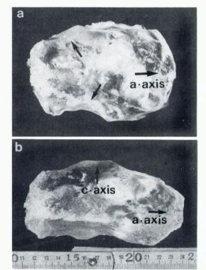
Fig. 2. Photographs of a large-sized single crystal of ice from Mendenhall Glacier with the crystallographic axes denoted by arrows; a: view from above; b: side view.
