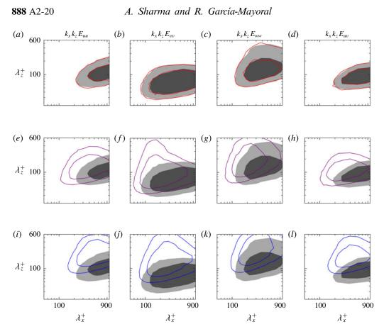
FIGURE 13. Premultiplied spectral energy densities at  $y^+ \approx 15$  normalised by their respective r.m.s. value. The line contours represent (a-d) case G10; (e-h) case G40; (i-l) case G100. The filled contours represent the smooth-wall case, SC. The contours in (a,e,i), (b,f,j), (c,g,k) and (d,h,l) are in increments of 0.075, 0.06, 0.07 and 0.1, respectively.
