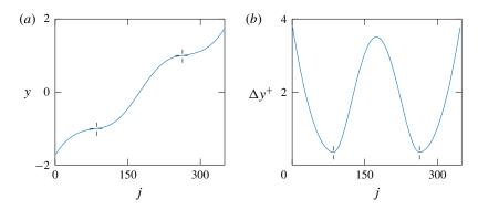
FIGURE 21. Wall-normal grid distribution for the simulation of case S10. (a) Variation of the wall-normal coordinate and (b) grid resolution with an equispaced auxiliary variable j. Dashed lines mark the location of the canopy tip plane.
