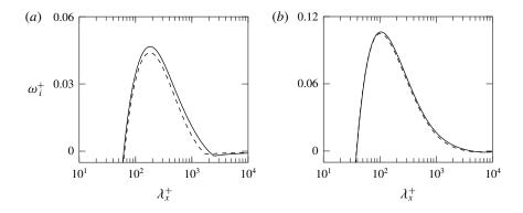
FIGURE 17. Growth rate for different perturbation wavelengths from the stability analysis for cases —,  $H32_{180}$ ; and ---,  $H32_{400}$ ; (*a*) with drag and (*b*) without drag on the perturbations.
