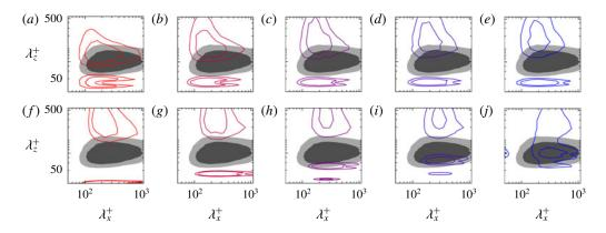
FIGURE 11. Premultiplied spectral energy densities of the wall-normal velocity,  $k_x k_z E_{vv}$ , for (a-e) cases H16 to H128 at a height of  $y^+ \approx -10$ ; and (f-j) cases S10 to S48 at a height of  $y^+ \approx -40$ . The contours are normalised by the r.m.s. values of their respective cases. The shaded contours are of the smooth-wall case, SC at a height of  $y^+ \approx 1$ , for reference. The contours are in increments of 0.075 for all the cases.
