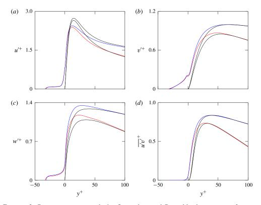
FIGURE 3. Root mean square velocity fluctuations and Reynolds shear stresses for cases H32<sub>180</sub> in red and H32<sub>400</sub> in blue. The black lines represent the corresponding smooth-wall cases. The data for the smooth-wall simulations at  $Re_{\tau} \approx 400$  are taken from Moser, Kim & Mansour (1999).
