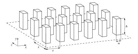
FIGURE 2. Schematic of the canopy layouts considered in the present study. The canopies are characterised by their element height, h, the element width, w, and the element spacing, s. Note that the elements have a square top-view cross-section.
