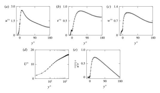
FIGURE 22. Root mean square velocity fluctuations, mean velocity and Reynolds shear stress profiles. The solid lines represent the results obtained from the present code, and the + symbol represent the data of case C12 from Abderrahaman-Elena *et al.* (2019).
