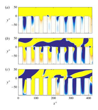
FIGURE 20. Instantaneous realisations of the (a) streamwise, (b) wall-normal and (c) spanwise velocities in a plane passing through the middle of the canopy elements for case S48, scaled with the friction velocity  $u_{\tau}$ . The clearest and darkest contours represent intensities of  $\pm 0.1$ , respectively.
