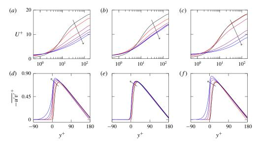
FIGURE 9. Profiles of the (a-c) streamwise mean velocity and (d-f) Reynolds shear stresses. The lines from red to blue, indicated by the direction of the arrows, represent (a,d) cases S10 to S48; (b,e) cases H16 to H128; and (c,f) cases G10 to G100. The black lines represent the smooth-wall case, SC.
