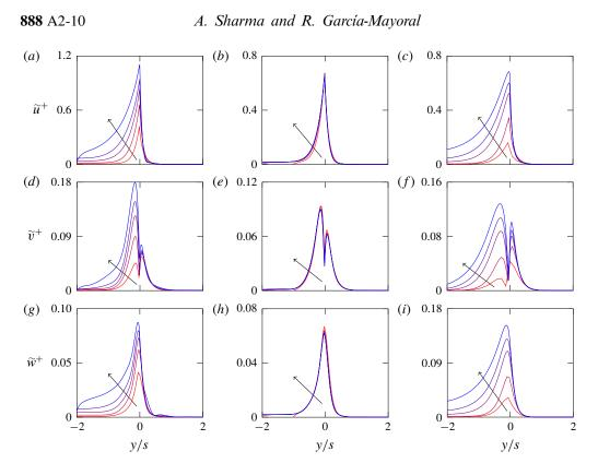
FIGURE 6. Root mean square velocity fluctuations of the element-induced flow. The lines from red to blue, indicated by the direction of the arrows, represent (a,d,g) cases S10 to S48; (b,e,h) cases H16 to H128; and (c,f,i) cases G10 to G100.
