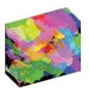
The 3D-OMiTEM produces 3D orientation maps from electron-transparent specimens that are substantially thicker than the average grain size. Existing 3D electron backscatter diffraction (3D-EBSD) techniques require destructive serial sectioning of the sample as part of
